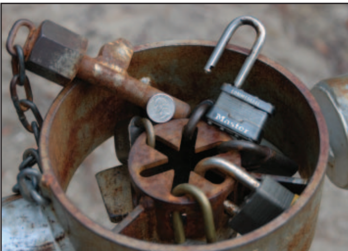
A 6-lock gate design. The removal of one lock allows the heavy-duty pin to be pulled from the housing to open the gate. The pipe tube in which this mechanism is located makes it difficult to manipulate bolt cutters to the locks.
