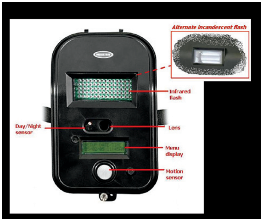
Basic components of a digital scouting camera (Moultrie® Game Spy™ I-40 and inset of an M-40). Credit: Moultrie® website ( www.moultriefeeders.com ) with labels by Anna H. Smith
