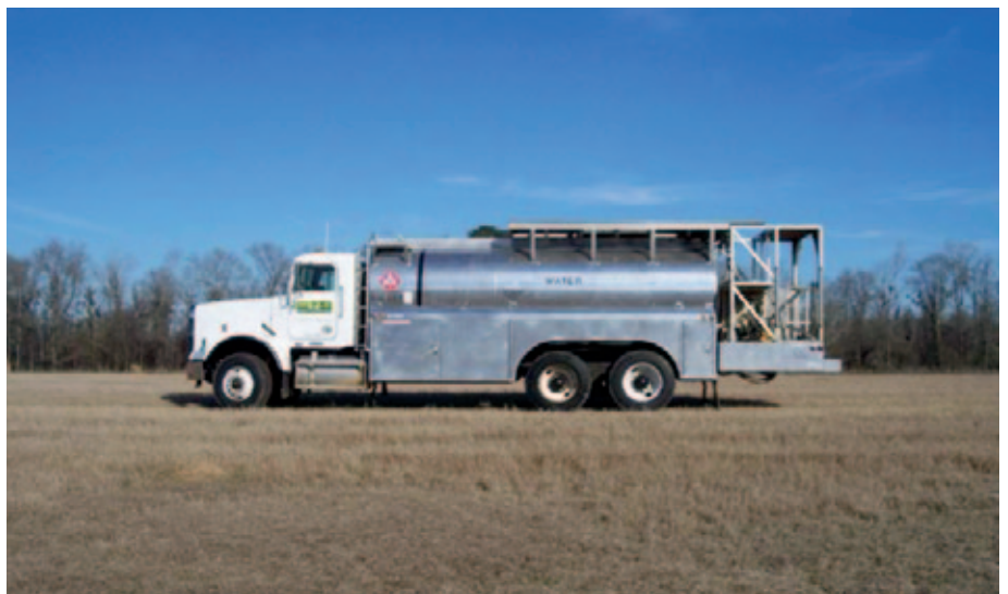
The batch truck is where the pilot receives the herbicide load and fuel. The helicopter lands on the platform on top. Note the limited clearance and weight. Good roads always helps the crew.
