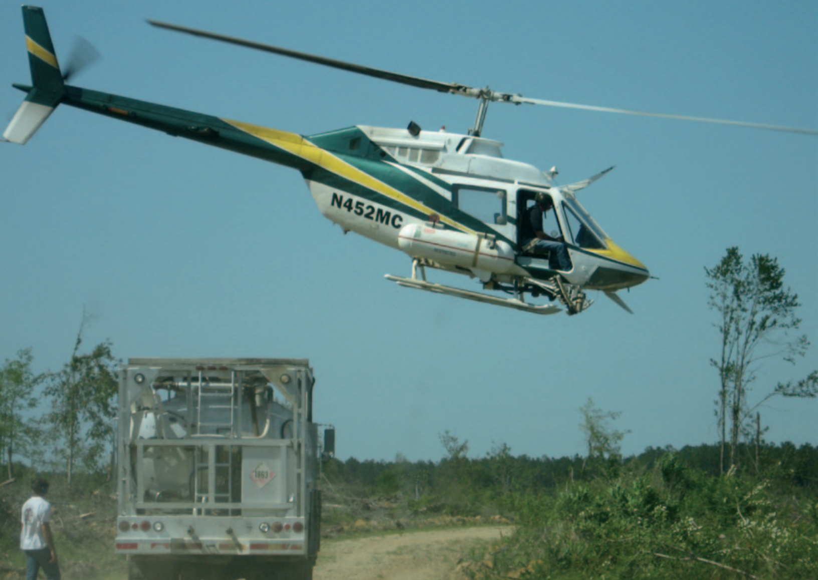
This is the sink effect the helicopter makes after leaving the top of the batch truck fully loaded. This is why we need plenty of clearance so the pilot can have a 'runway' to begin the lift. Photo courtesy of Robert Sullivan.
