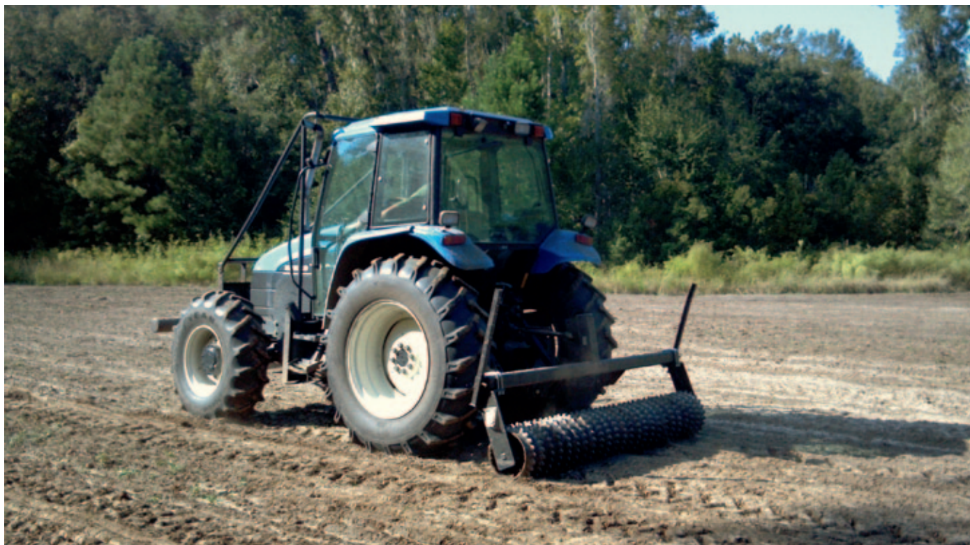
A cultipacker is a great implement for smoothing food plots and “packing” seed once planted
