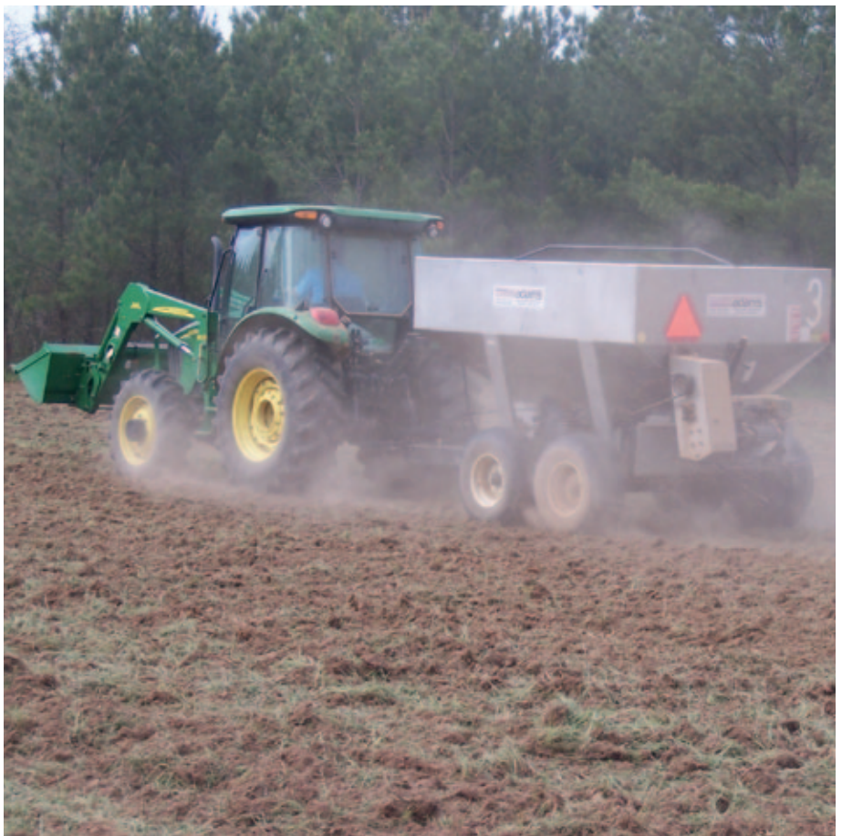
Renting a fertilizer buggy is inexpensive and allows you to efficiently apply bulk fertilizer more quickly and effectively
