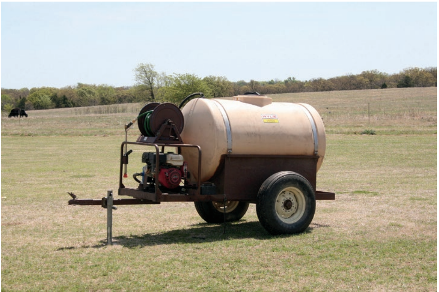
This is a 250 gallon sprayer equipped with a broadcast spray nozzle in the back and a hand wand/gun. It is used to spray pastures and fence lines as well as during prescribed burns.
