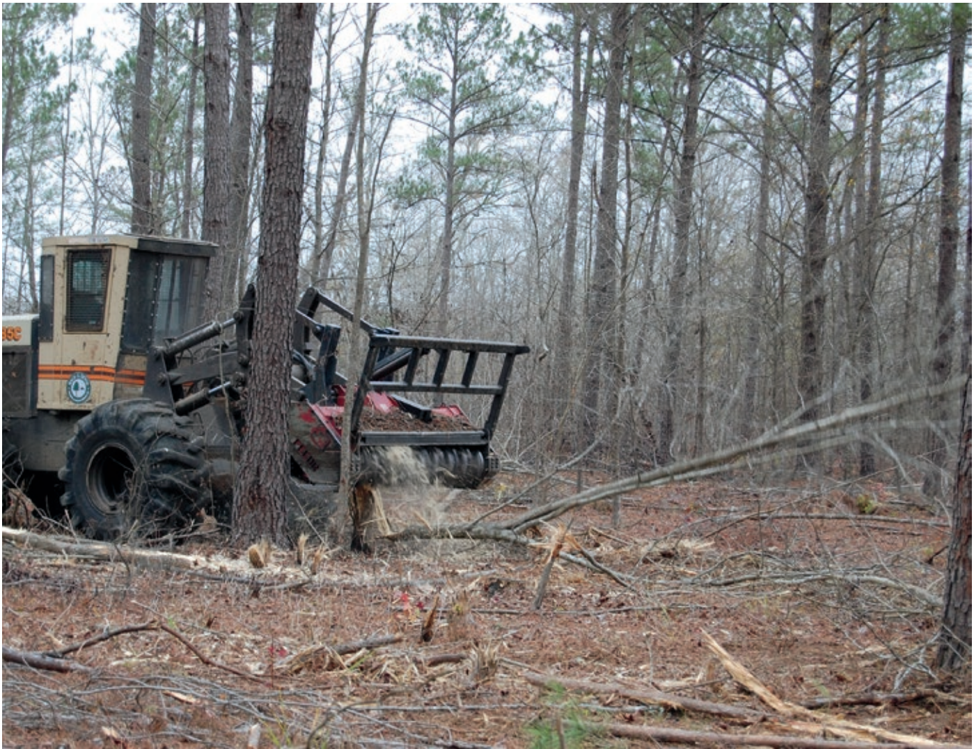
Mulchers are often used to follow up behind thinning jobs and logging crews to “clean up” the look.
