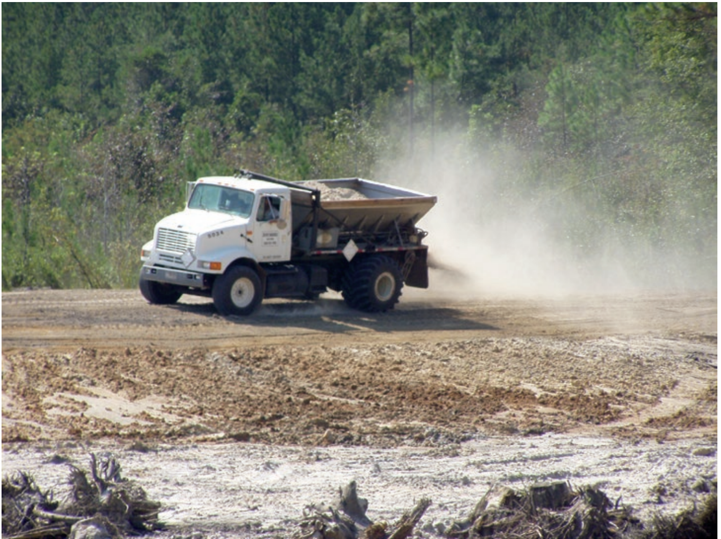
It is much easier to spread lime in a lake bottom before refilling than using a boat after water is present.
