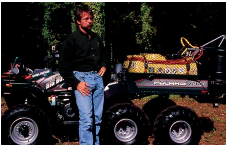
Polaris Big Boss 500 6X6 rigged with two 25-gallon spray tanks in back, Model 045 BoomBuster® nozzles, and two Moultrie seeders.
