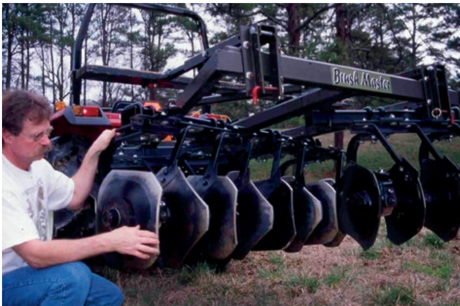
Amco Brush Master® with square discs. Disc gangs are attached with flex risers that absorb shock when discing over stumps. Scraper blades keep the discs clean. The drag board smoothes the soil behind the disc.
