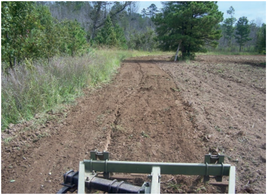
Brush Master® with drag board down, which levels and smooths the soil. Note the well established ecotone around the field. This is the second pass.
