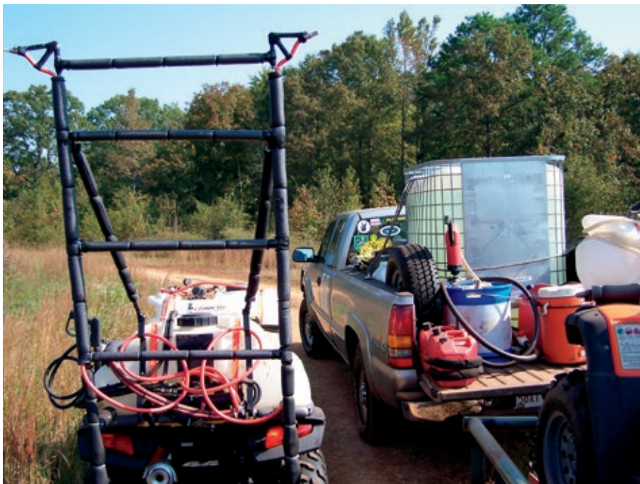
Flex boom with two Model 045 BoomBuster® nozzles. Spray 18' per side, with about 4' overlap behind the ATV, for a swath width of about 40'. Note the 335 gallon mix tank.
