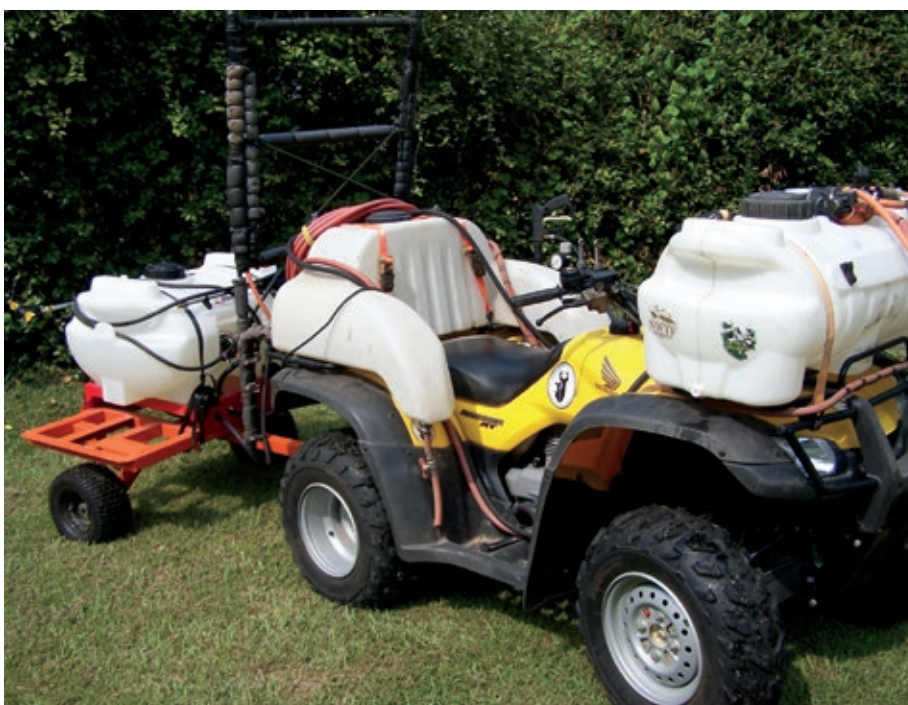
ATV configuration utilizing two 25-gallon tanks and a 50-gallon pup trailer, for a total capacity of 100 gallons, capable of spraying 10 acres @ 10 GPA/load. Note flex boom.
