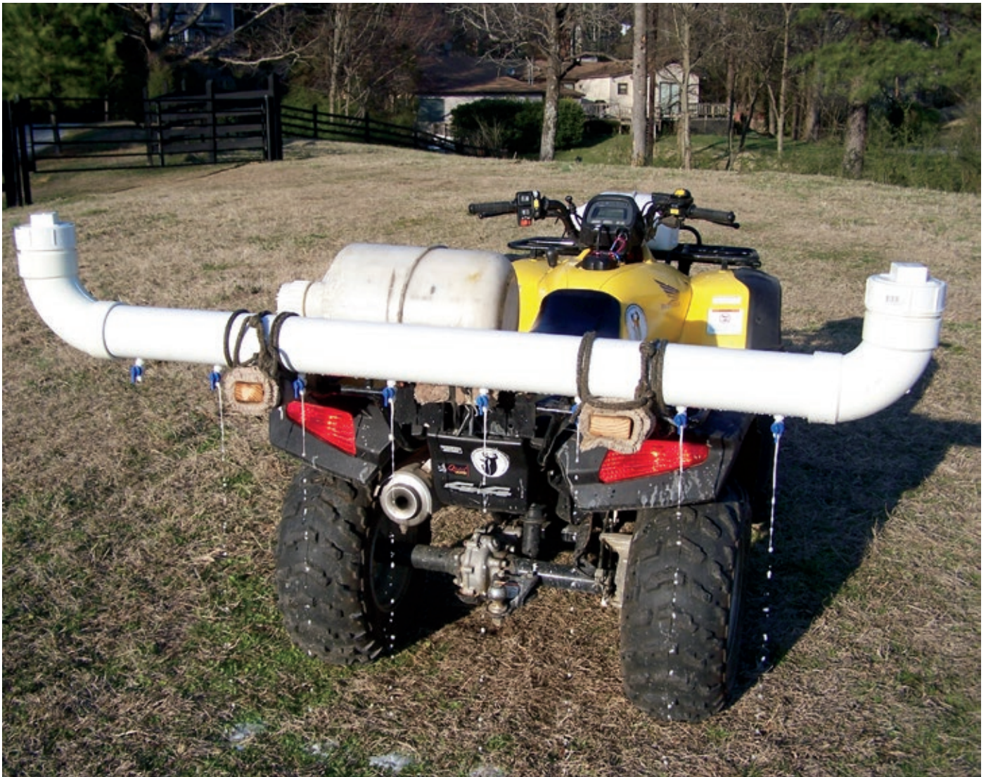
This is my liquid lime dispenser, made from PVC pipe, for liming smaller food plots. Works great.
