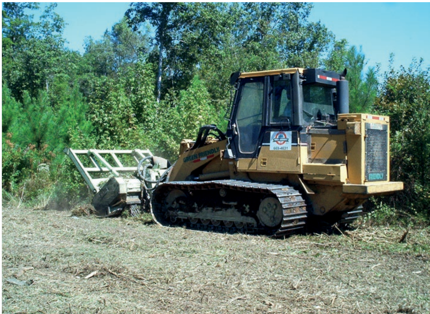
Summer is a great time to create new food plots or expand existing ones. A forestry mulcher is an efficient machine for land clearing.
