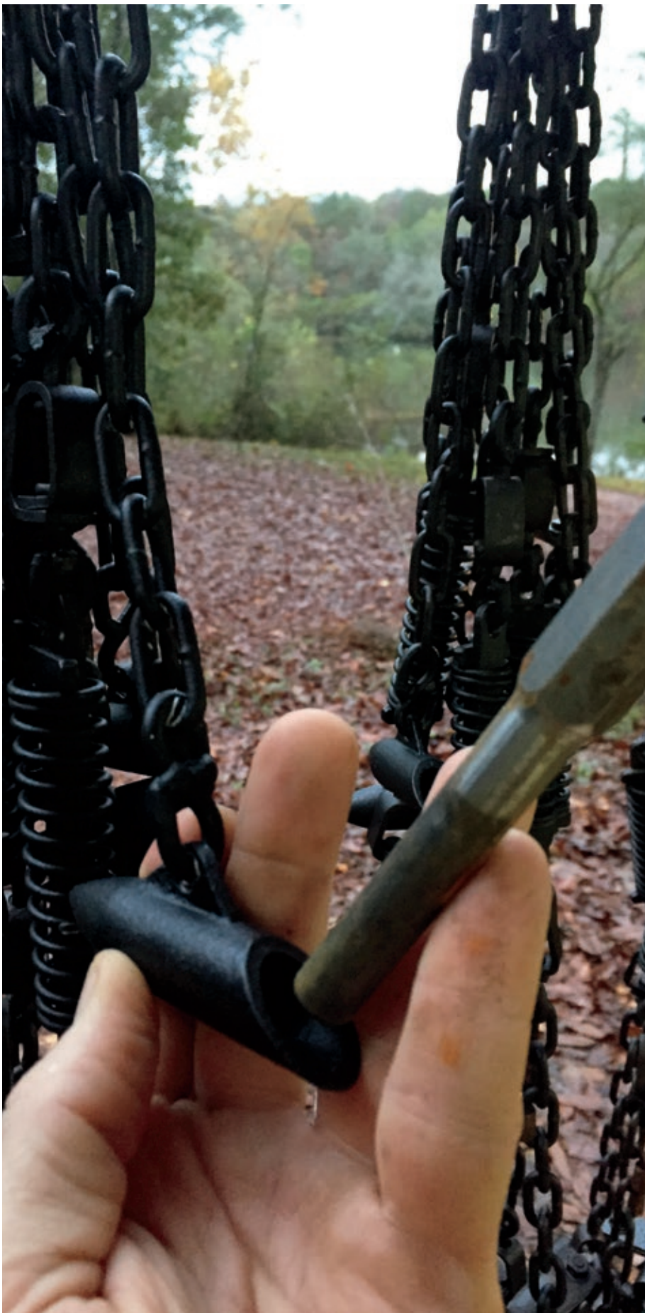
An independent anchor such as the Fox Hollow version provides a steadfast anchoring system. Shown here with the terminal end of the driver.
