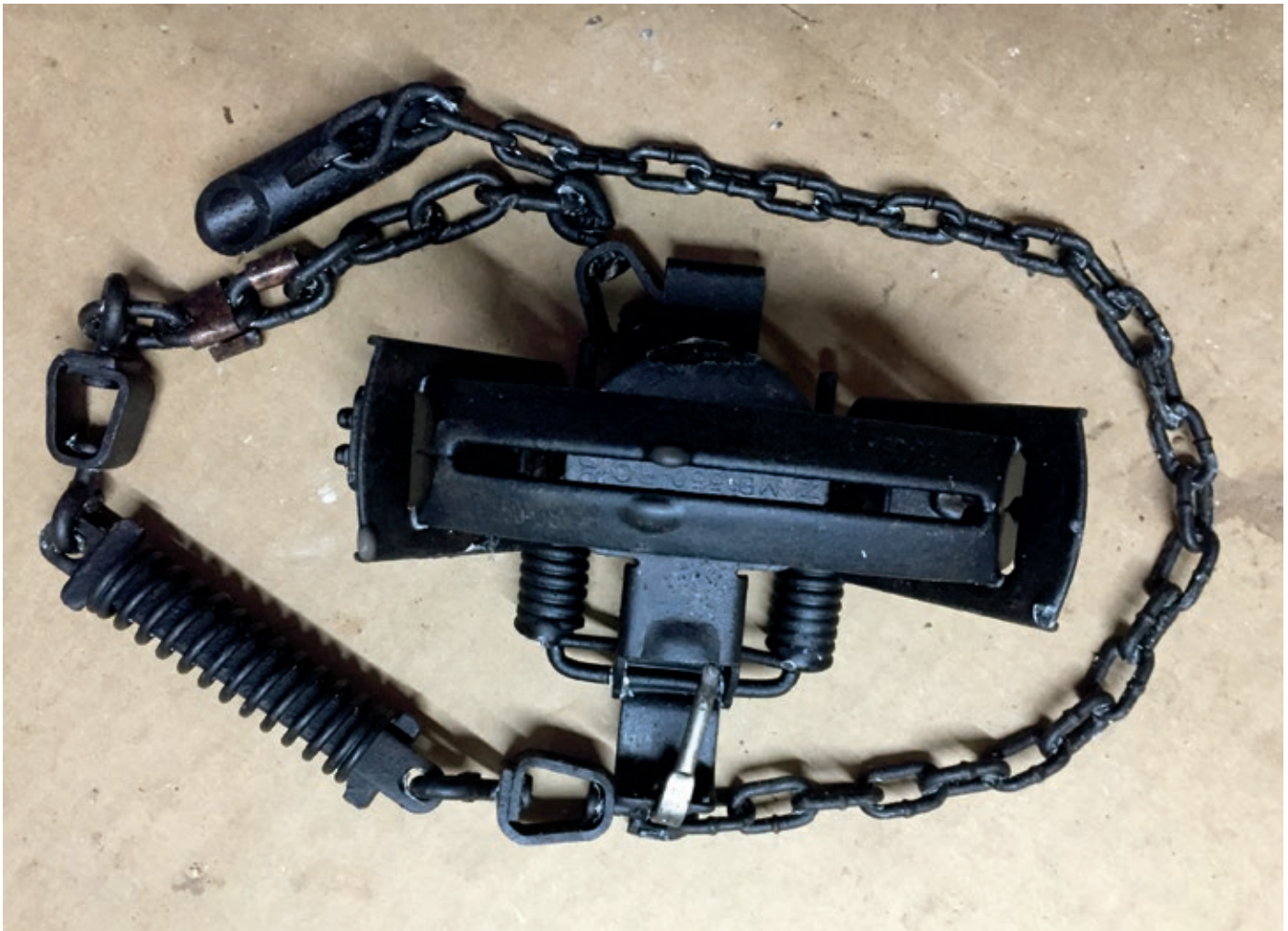
A modern-day foot-hold trap, MB550. Note the 3 swivels, shock spring and offset jaws that make for an efficient and humane trap.
