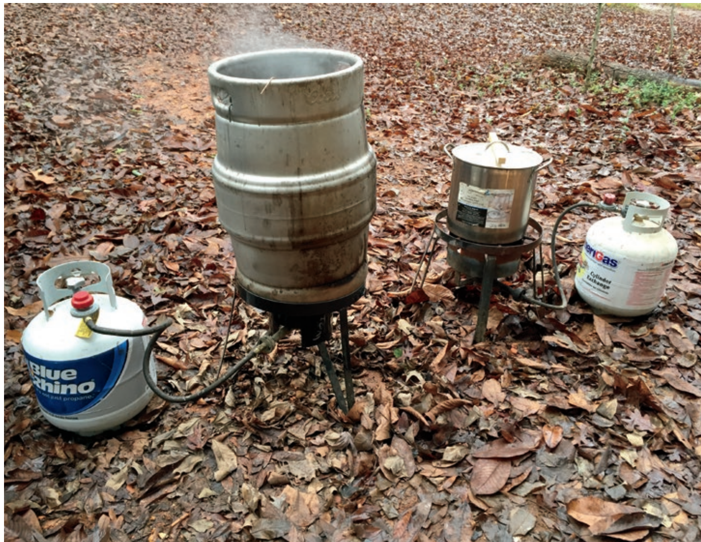
The arrangement can effectively dye an abundant amount of traps in an afternoon. A converted keg for the dye and a smaller pot for the wax serve this purpose well.
