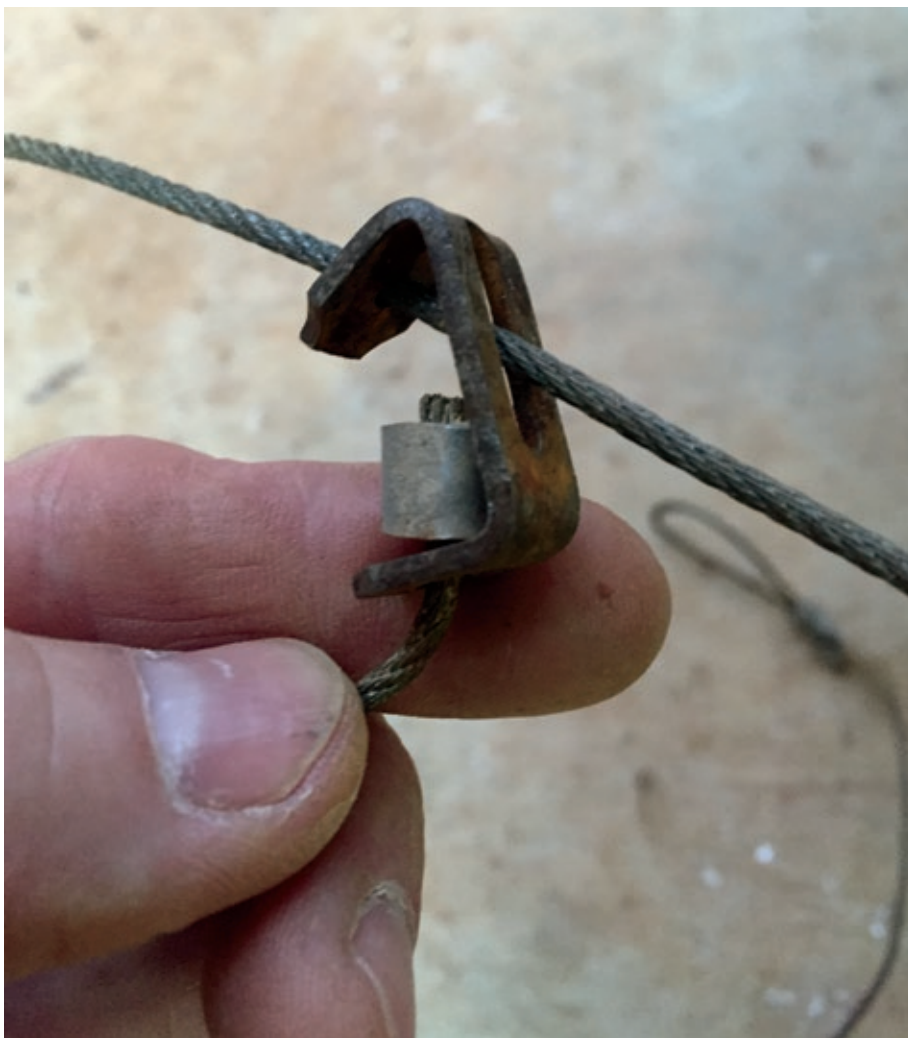
Locking device designed to close and hold the loop of the snare.
