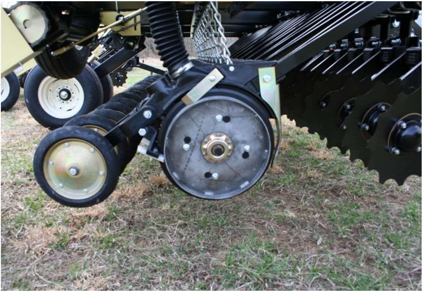
Native Drill showing openers and depth bands.
