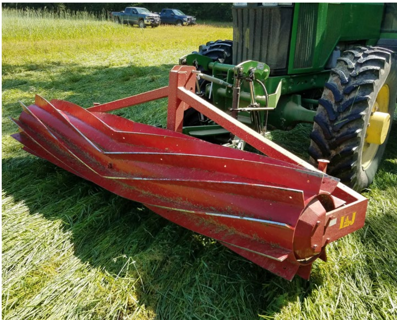
The buffalo of the future, a roll crimper. The roll crimper will roll and flatten the vegetation, while the crimper (blades) will crimp plants to terminate plant function. No need for herbicides.
