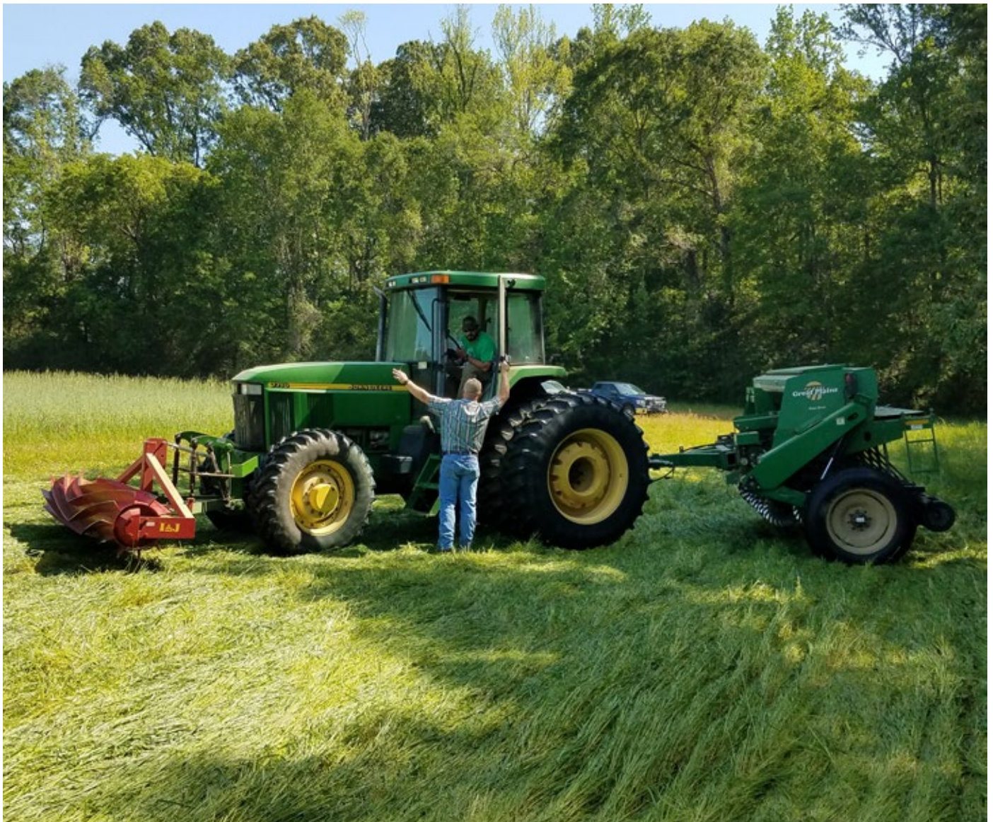
One tractor pass system. Roller Crimper on front and No-till Drill in back. Most efficient way to plant.
