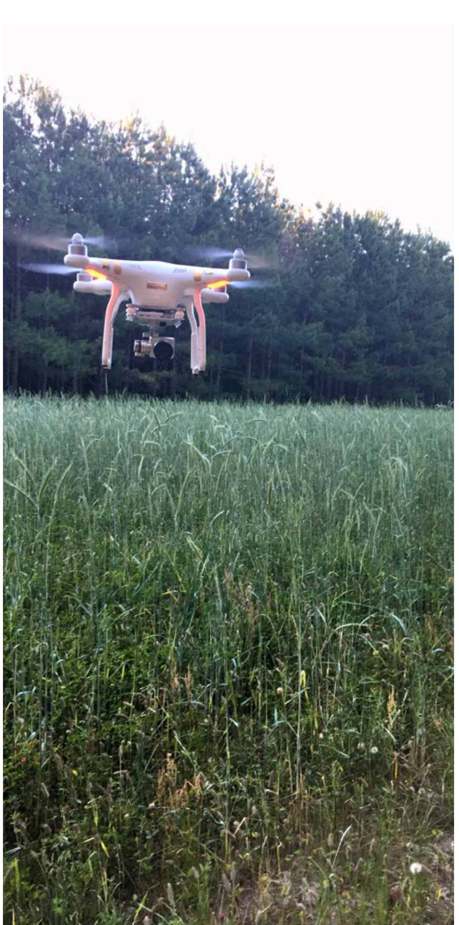
The camera on most drones has a wide angle, fixed power lens. In order to get close-up shots you have to position the aircraft close to the subject. This is useful when inspecting fields or food plots for damage from hogs, insect pests, weeds or disease.
