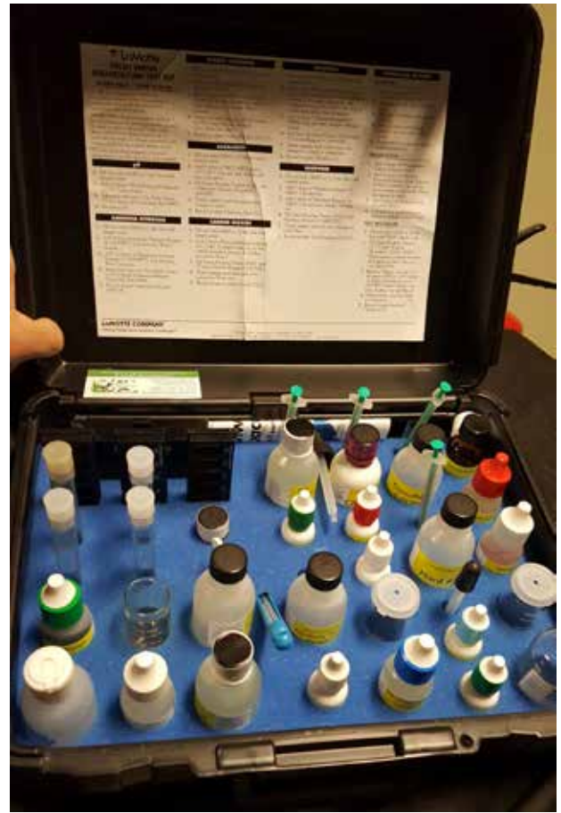
Water chemistry is the foundation of any lake management plan. This kit tests most parameters a lake manager is concerned about and costs considerably less than electronic meters.
