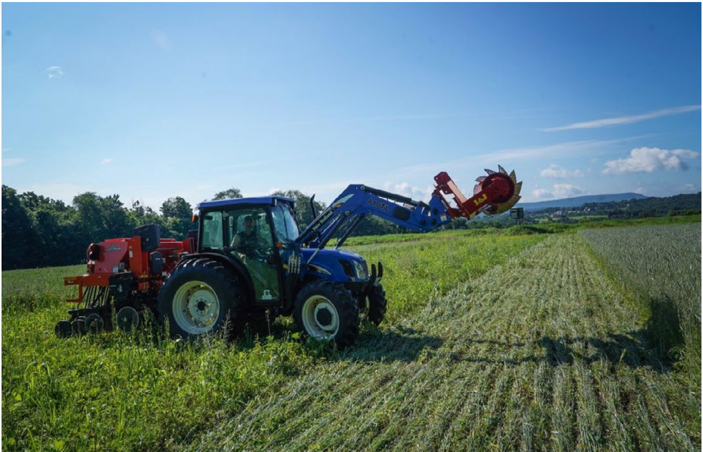
With a single pass, the author can simulate running a herd of Bison across the pasture and drill a season-specific, diverse cocktail blend. This efficient system eliminates the need for tillage, fertilizer, herbicide and reduces fuel costs with a single pass across the field.
