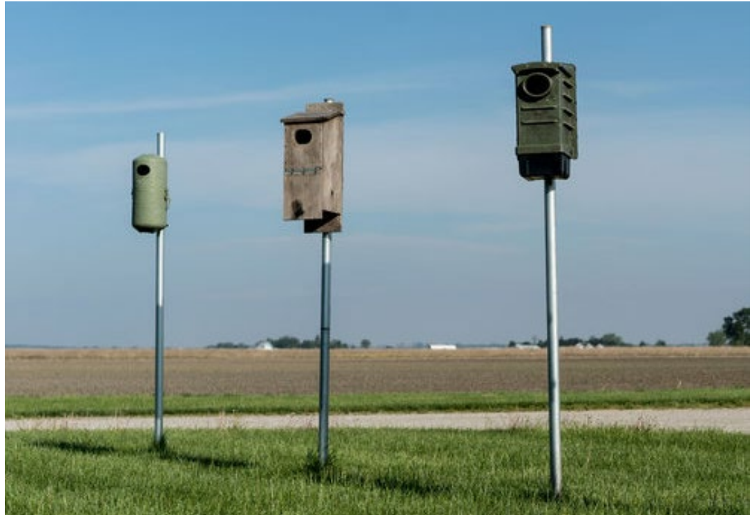
Figure 2. DuckHut temperature test site, Wapello, IA July 16-26, 2016. Three different nest box materials (plastic, wood and metal) were compared.
