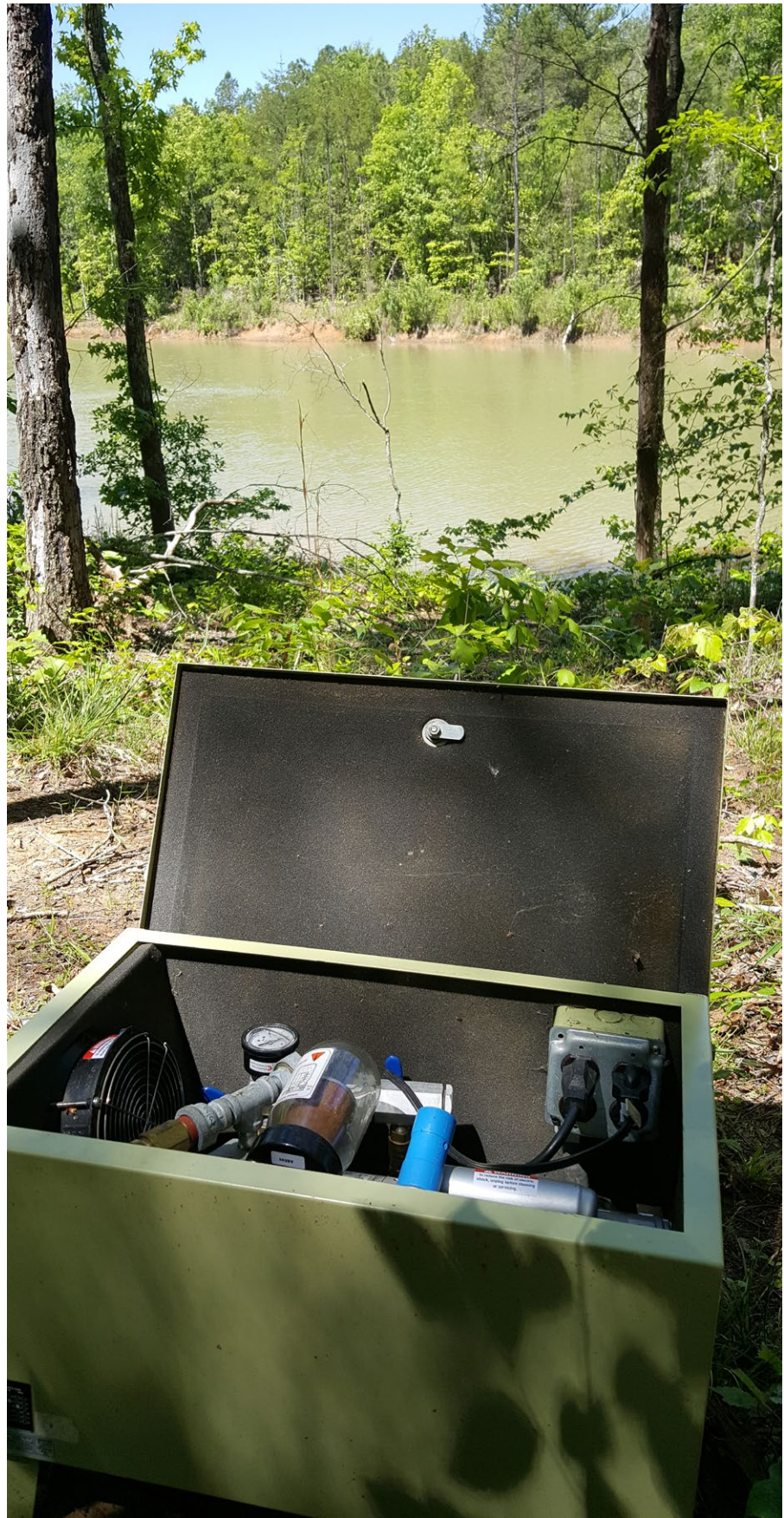
This is a very young pond, only a few years old, with an algae bloom fed by surrounding agriculture and an aeration system that maximizes the carrying capacity.
