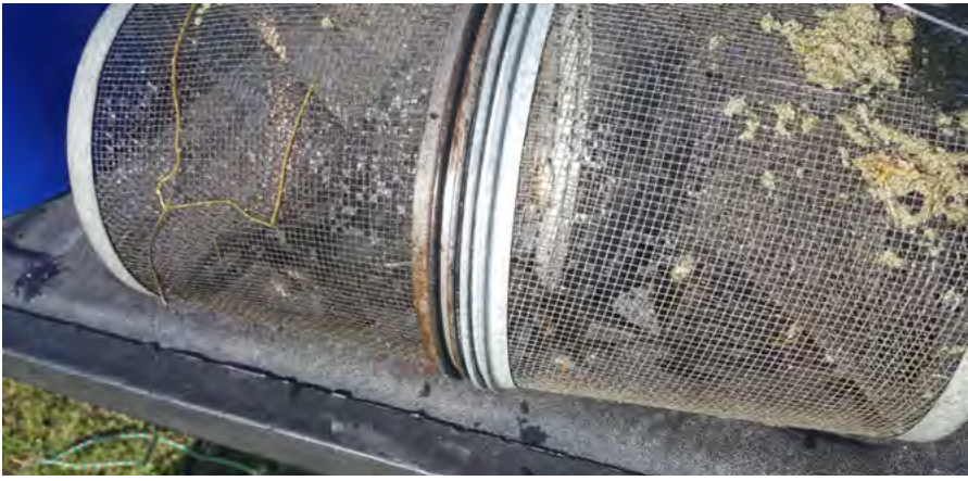
Sometimes the common minnow trap is overlooked as a sampling tool or fish collecting device. Although it collects small individuals, baited it works well collecting small bream, mosquitofish and golden shiners.
