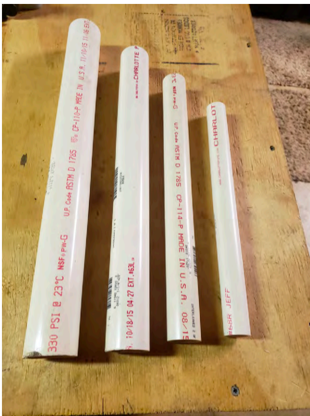
Standard set of PVC tubing for checking largemouth bass stomachs. This set is not completed as the end has not been beveled to reduce harm to the fish.
