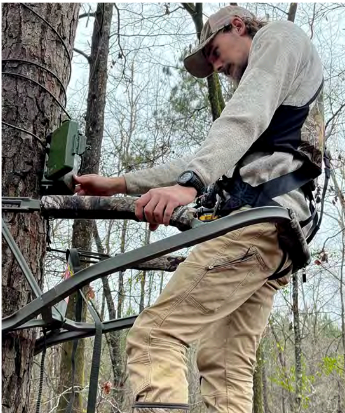
Matt Day uses a climbing treestand to place ARU's above the reach of someone standing on the ground to prevent theft. Climbers are also used to check battery levels and exchange SD cards on a regular basis. Photos by Tess Randle Jolly.
