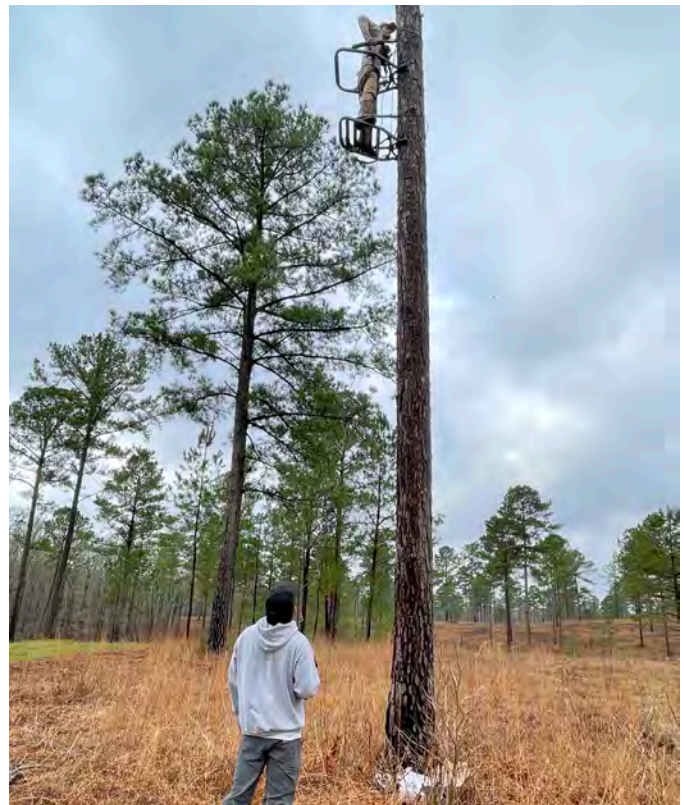
Matt Day uses a climbing treestand to place ARU's above the reach of someone standing on the ground to prevent theft. Climbers are also used to check battery levels and exchange SD cards on a regular basis. Photos by Tess Randle Jolly.
