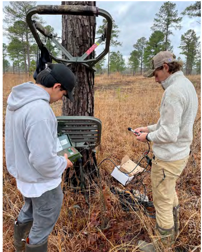
Matt Day and George Goto program specific start and stop recording times into ARU's to capture audio during likely gobbling periods over a two month period. Photo by Tess Randle Jolly.
