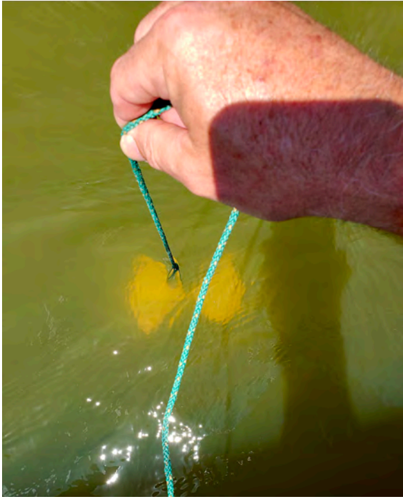
Checking visibility about every two weeks with a Secchi Disk is mandatory once a fertilization program is initiated. This water looks pretty good and is probably in the desirable zone of 18-36 inches.
