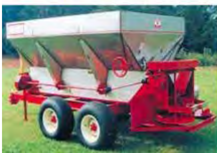
A fertilizer spreader equipped gravity-fed bin, a chain to pull grain, and spinners to sling feed is the most common method of broadcast distribution of supplemental feed.
