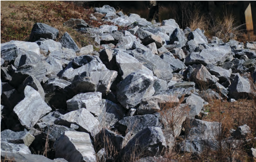
Many habitat improvements are easier done when the lake is dry. This riprap will secure a shoreline prone to erosion and provide hiding for small fish and crawfish.
